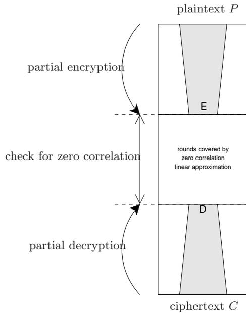
**Fig. 7.** High-level view of key recovery in zero correlation linear cryptanalysis
