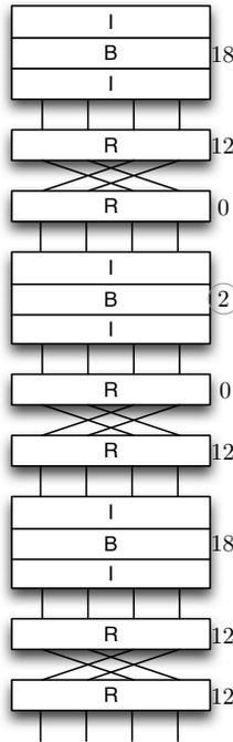
**Fig. 23.** Partial matching over 3 rounds for SC2000: Numbers indicate the number of S-boxes to be recomputed in the corresponding functions ( $B$  or  $R$ ). The number in grey circle indicates the point of matching
