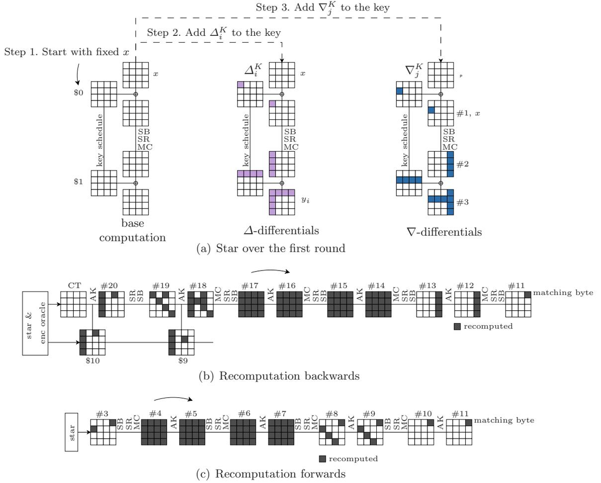
**Fig. 9.** Fastest biclique attack on AES-128 with minimum data: time  $2^{126.7}$  and data 1 or 2 KPs
