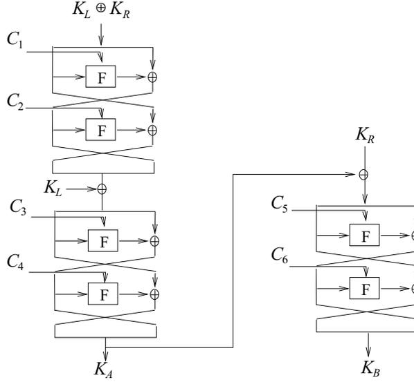
**Fig. 16.** The Calculation of  $K_A$  and  $K_B$
