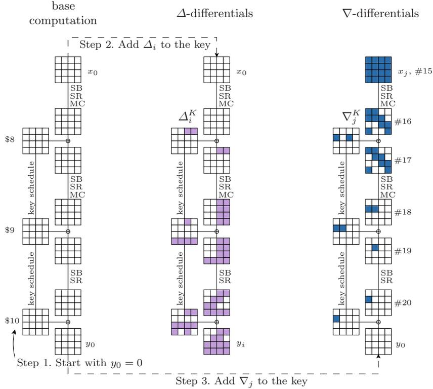
**Fig. 6.** Biclique over 3 last rounds of AES-128 from independent differentials [13]
