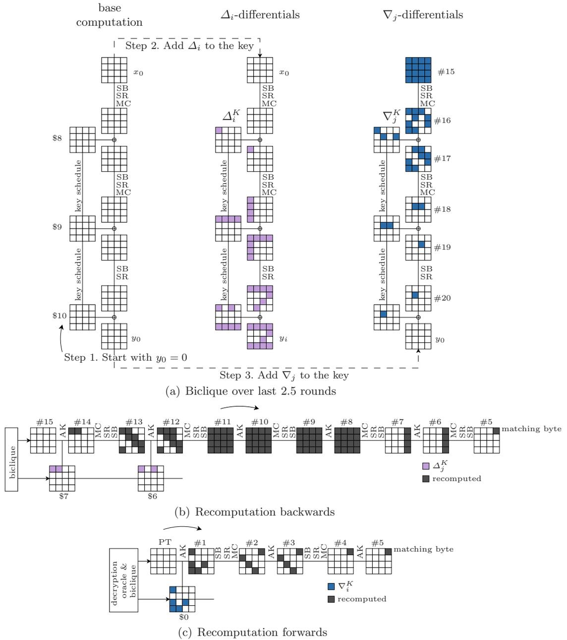
**Fig. 10.** Fastest biclique attack on AES-128 with less than full codebook: time  $2^{126.16}$  and data  $2^{64}$
