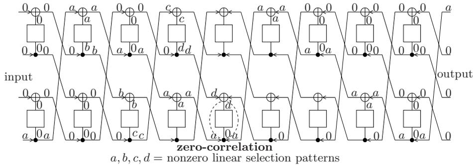
**Fig. 19.** 9-round zero-correlation linear approximation for CLEFIA-type ciphers (type-II generalized Feistel network) with balanced F-functions
