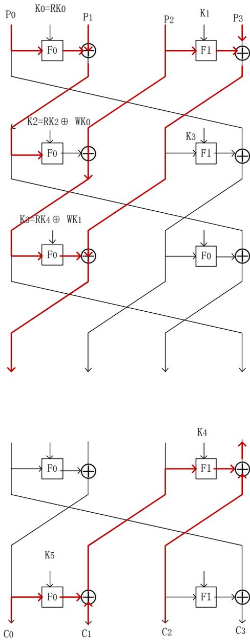
**Fig. 22.** Zero correlation linear attack on 14-round CLEFIA-256
