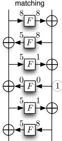
**Fig. 13.** Partial matching over 3 rounds for Camellia: Numbers indicate the number of bytes to be recomputed in the corresponding lines. The number in grey circle indicates the byte of matching
