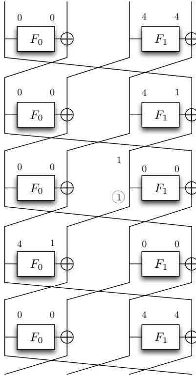
**Fig. 18.** Partial matching over 5 rounds of CLEFIA: Numbers indicate the number of bytes to be recomputed in the corresponding lines. The number in grey circle indicates the byte of matching
