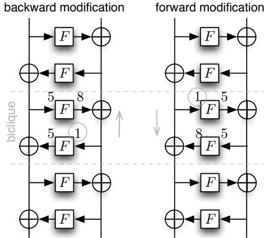
**Fig. 12.** Independent biclique construction over 2 rounds of Camellia: Numbers indicate the number of active bytes in the  $F$ -function right after the subkey addition and right after the  $P$ -layer. Numbers in grey circles indicate spots of key difference injections
