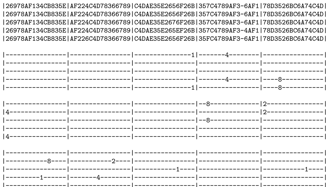
Fig. 57. A 3-round characteristic leading to a collision KECCAK-256 with probability 2^{-24} [22]. Note that the order of lanes is from left to right.
